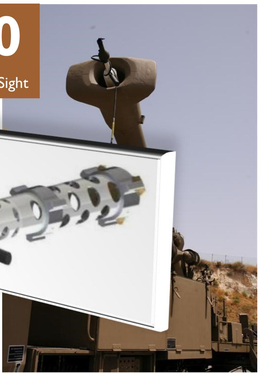
*Video Bore Sight (VBS) for all barrels. Enabling fast and easy calibration of gun sights, including image on the fire computer main screen or Stand-Alone Video Overlay Generator with screen*
